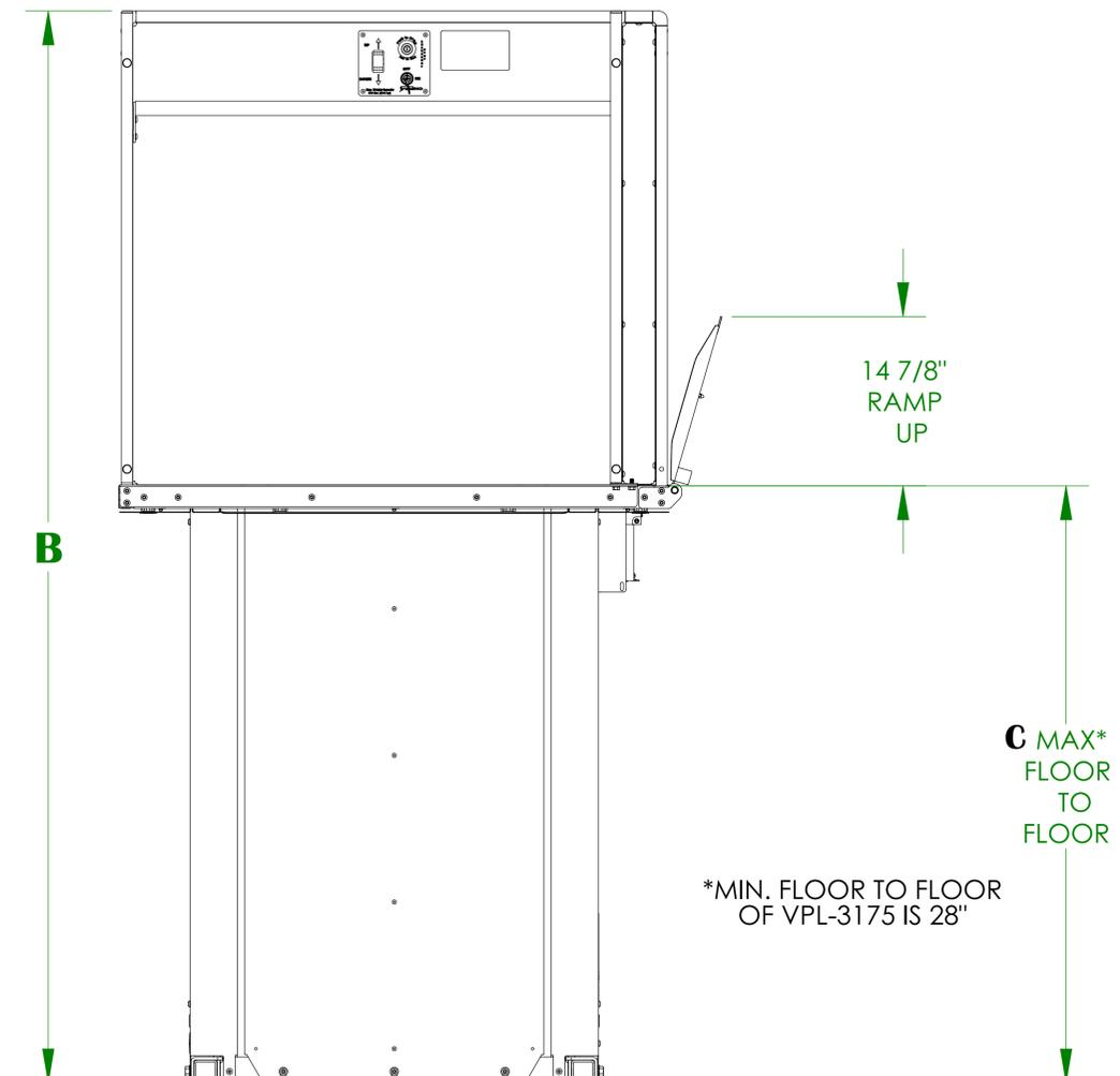
NOTES: 1) ACCESS RAMP CAN BE MOUNTED ON EITHER SIDE OF THE PLATFORM
